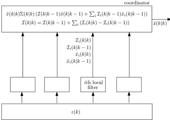
Figure 8.8: Distributed Kalman filtering with a coordinator
