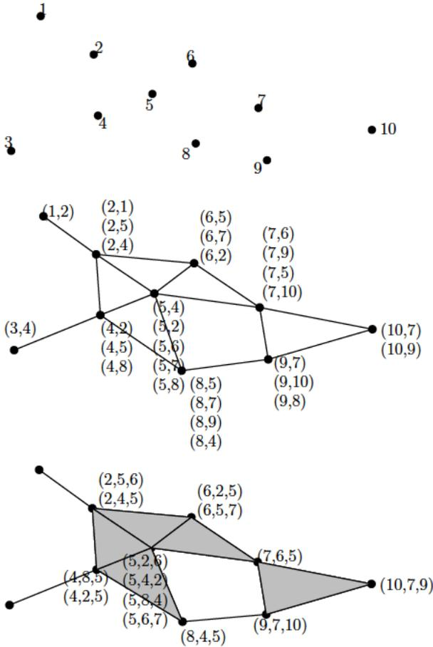
Figure 13.5: A decentralized protocol for obtaining the Rips complex. Using a broadcast protocol, the network discovers higher-dimensional simplices in the Rips complex  $\mathcal{R}$ . At each broadcast cycle, the information gathered from the previous broadcasts is sorted and passed on to neighboring nodes. The figure shows a progression from 0-simplices (top) to 2-simplices (bottom).
