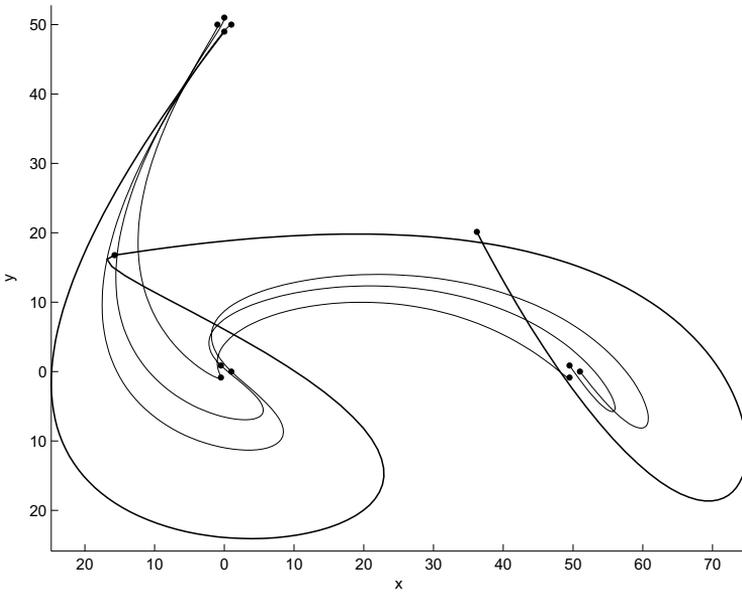
Figure 10.10: Starting at a formation close to  $(0, 50)$  at time  $t = 0$ , the leader (thick curve) maneuvers the followers to the new positions close to  $(0, 0)$  at  $t = 5$ , and close to  $(50, 0)$  at  $t = 10$ . This is done while expending the smallest possible control energy.
