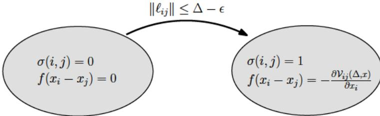
Figure 7.2: The hysteresis protocol for adding interagent tension functions to the total tension function only when agents get within a distance  $\Delta - \epsilon$  of each other, rather than when they first encounter each other at a distance  $\Delta$
