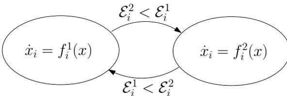
Figure 6.10: A hybrid automaton implementing the strategy in which agent  $i$  selects the dynamics  $\dot{x}_i(t) = f_i^1(x(t))$  over  $\dot{x}_i(t) = f_i^2(x(t))$  if  $\mathcal{E}_i^1 < \mathcal{E}_i^2$
