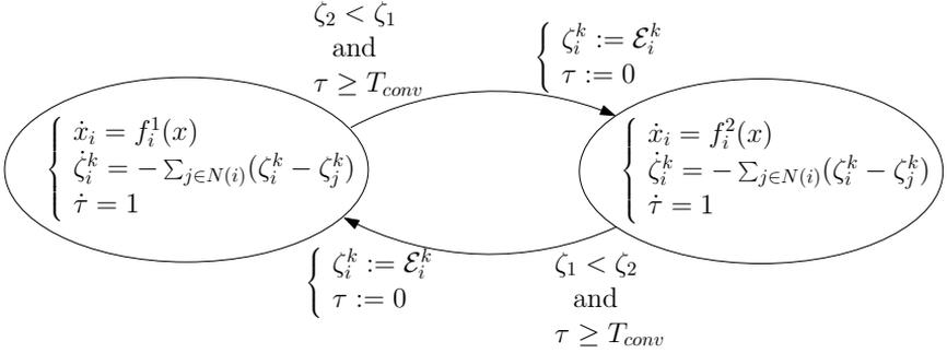
Figure 6.11: A transition between formations occurs when the guard conditions are met ( $\zeta_i^k < \zeta_i^\ell$  and  $\tau \geq T_{conv}$ ) at which point the states are reset to  $\zeta_i^k = \mathcal{E}_i^k$  (new error estimate) and  $\tau = 0$  (waiting time reset).
