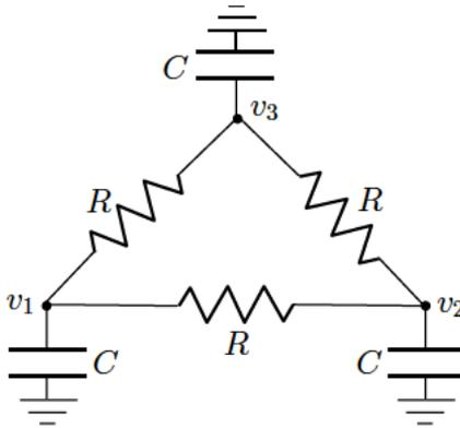
Figure 3.2: A capacitor-resistor network
