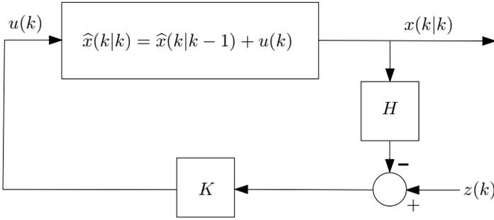
Figure 8.7: Kalman filter as a feedback mechanism
